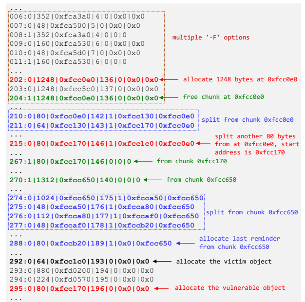
Figure 6: Exploitable heap trace record snippet for CVE-2017-14164. Each item is represent as four-tuples \langle op|size|addr|index \rangle where “1” means the deallocate operation while “0” represents the allocate operation. Each chunk contains 16 more bytes to record other information.
